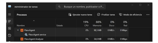
FlexxAgent consists of a Windows service called FlexxAgent Service, which manages two processes: FlexxAgent (process), which runs at the system level, and FlexxAgent Analyzer (process), which starts for each user session.
